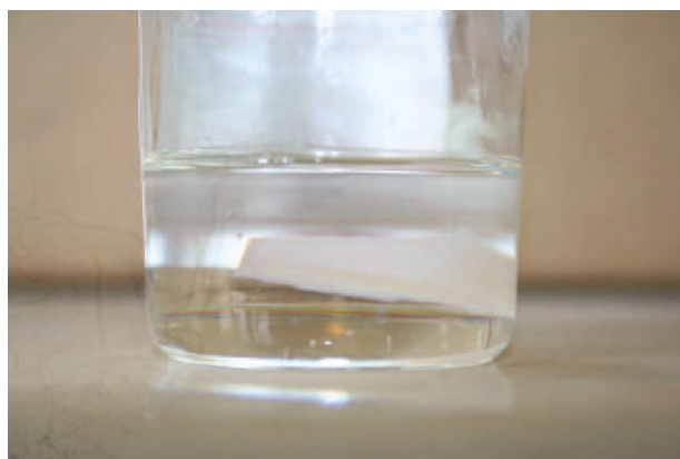
Figure 13 Photograph of the sample with 40 phr MDMA curing for 15 min swell in the mixture of toluene and chloroacetic acid once again for 72 h. [Color figure can be viewed in the online issue, which is available at wileyonlinelibrary.com .]
